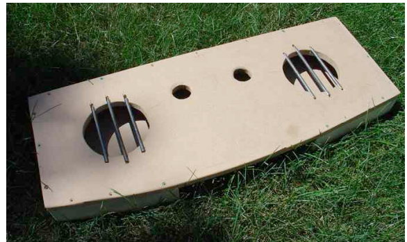
This illustration shows the solid construction of the speaker box. The baffle board averages more than a foot deep and almost three feet wide, offering a vastly superior mounting for speakers compared to any other options I could accommodate.
