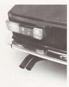
Twin exhausts produce that throaty six-cylinder sound without shattering the neighbors' windows. Wrap-around tail lights ensure visibility and set off the neat, square lines of the rear panels. Back up lights are standard.
