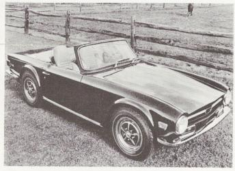
The TR-6 has a handsome new body styled by Karmann-Ghia, wider wheels and a front anti-sway bar for stability and a redesigned cockpit for increased driver comfort and convenience. Red-band radial tires are standard.
