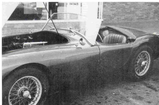
Bob Stanton of Binghamton, New York, put a Triumph engine in this AC Ace and claims higher performance and better reliability.
