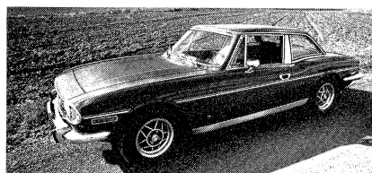
The 1973 Stag, last to be imported, had GKN five-spoke cast wheels and smaller, adjustable head rests. A side stripe was added.
