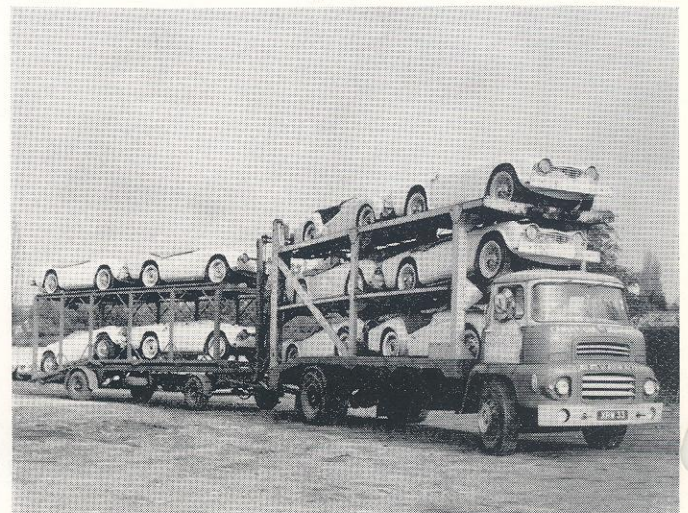
Believed to be one of the largest vehicles of this type in the world, this Leyland truck can carry 10 Triumphs at one time. Standard-Triumph International is a member of the Leyland group.
